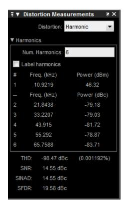
The harmonic distortion measurement automatically locates the largest sinusoidal component (fundamental signal frequency). It then computes the harmonic frequencies and power in each harmonic in your signal. Any DC component is ignored. Any harmonics that are outside the spectrum analyzer's frequency span are not included in the measurements. Adjust your frequency span so that it includes all the desired harmonics.
