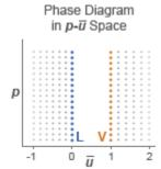
A pressure vector, of length N, and two normalized internal energy vectors, of lengths  $M_{\rm L}$  and  $M_{\rm V}$ , provide the  $(p, \bar{u})$  coordinates of the two grids. The pressure vector is common to both grids. The subcooled liquid grid is  $M_{\rm L}$ -by-N in size and the superheated vapor grid  $M_{\rm V}$ -by-N.
